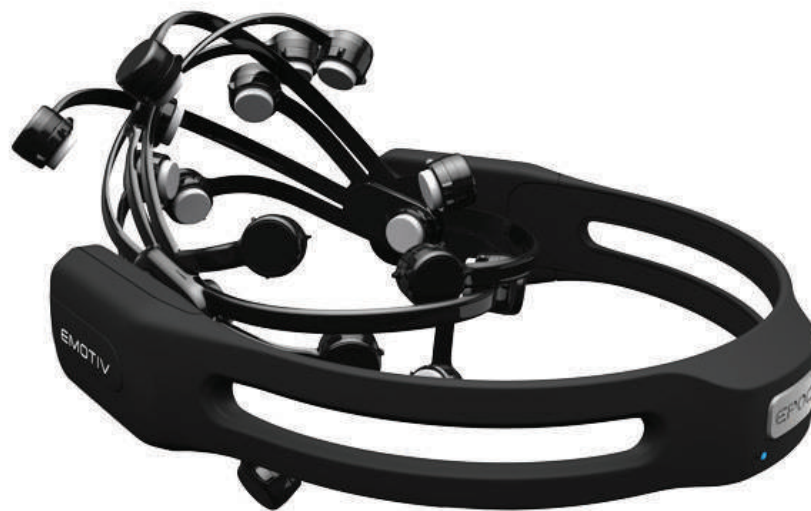
Emotiv Epoc + hi-resolution 14 channel mobile EEG headset
